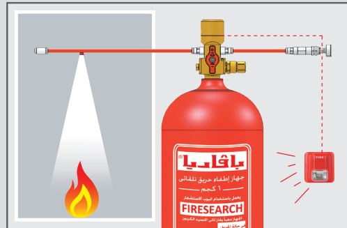
Direct Pressure Operated System
